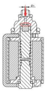
Solenoid valve malfunction: when closed, air is still flowing in as indicated by the arrow.
